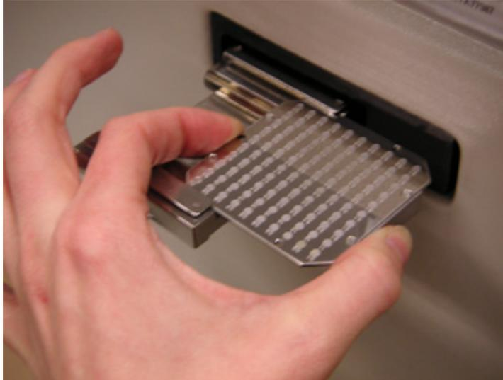
**Make sure orientation is correct!! See image below!! As you stand facing the instrument, sample spot #01 should be on the “south-east” corner, i.e. to the right and closest to you.**
