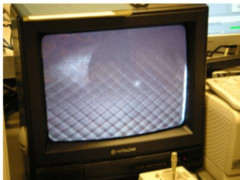
If there is no plate in the instrument, the monitor will show an empty sample stage:
