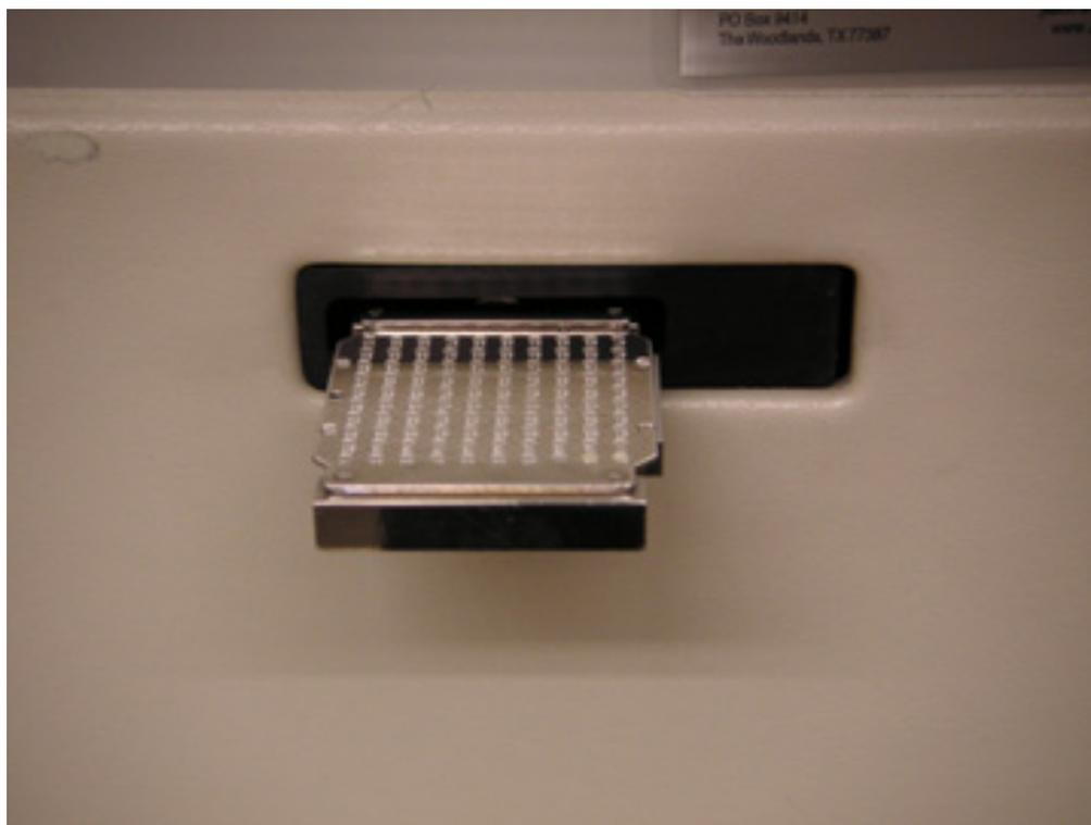
***NOTE: Do not leave the sample holder in the Eject position for more than a few seconds. Minimize the time the instrument is exposed to the atmosphere to reduce the time needed to reach high vacuum when you insert a new plate.***
