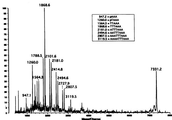
**Figure 1.** 24mer oligodeoxynucleotide TAAAGTTACTTTTCAAAATT-TAAA: a quasi-molecular ion  $[M-H]^-$  can be seen at  $m/z$  7331.2 (calc. 7331.9); below  $m/z$  3200 by-products from incomplete synthesis and deprotection steps are observed. The table lists the assignments of their phosphorylated peaks; the peaks 80 daltons lower are the unphosphorylated equivalents.
