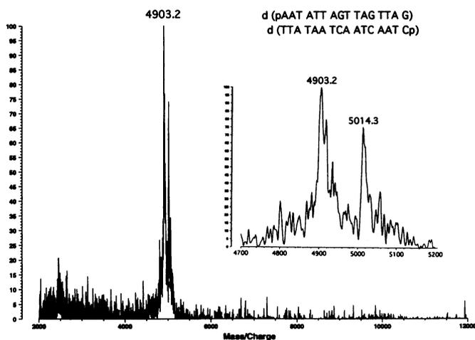
**Figure 2.** MALDI spectrum of a blunt ended double-stranded DNA fragment 16 bp (Sigma catalog # S 9650): the inset shows the two well resolved single strands.
